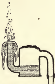
Fig. 276. Effect of Back Pressure.
